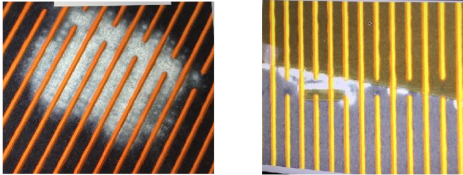
Figure 7.20: Zoomed pictures of a SM1 M3 readout panel after a three months irradiation period at GIF++. Visible are discharge residuals at strip interconnection zones (left) and close to the HV distribution line covered by a piralux coverlay (right).
