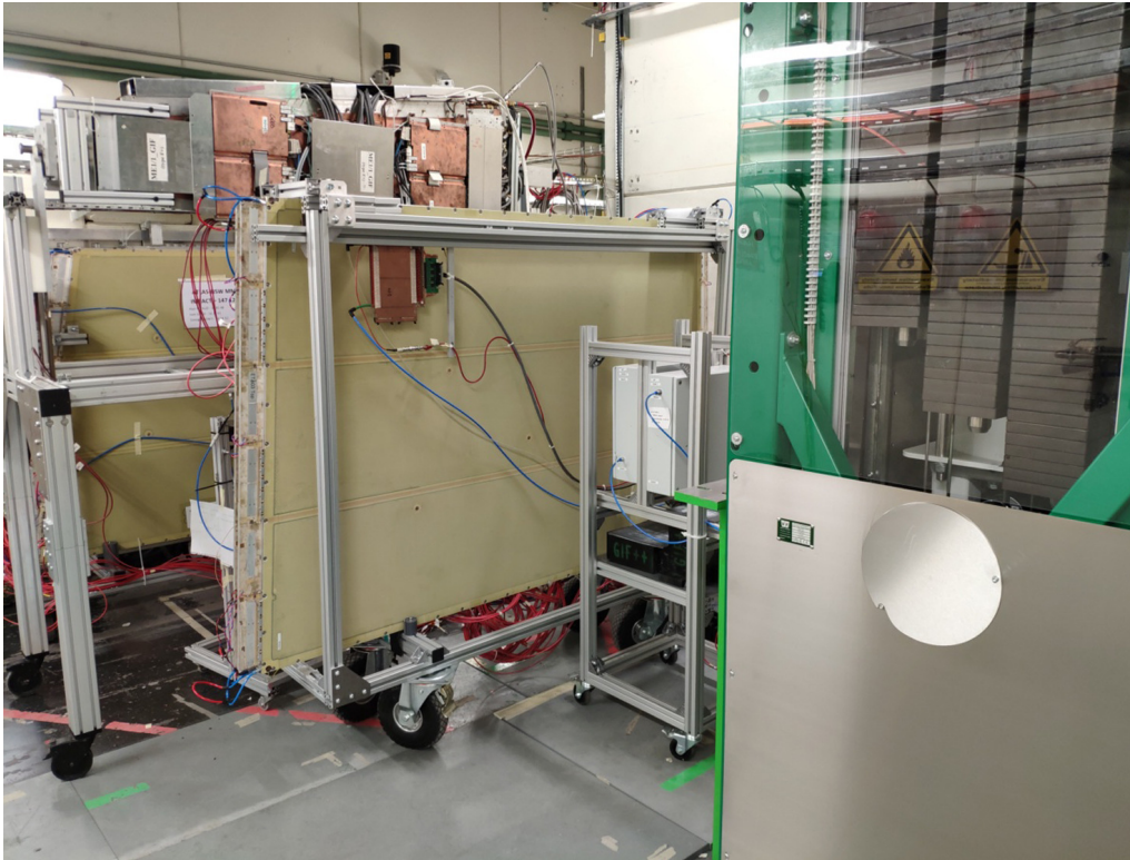
Figure 7.16: Picture of the LM2 M7 Micromegas chamber in the GIF++ bunker and the auxiliary TGC chamber mounted next to it. In the picture right side the GIF++ radiator wall is visible as well.
