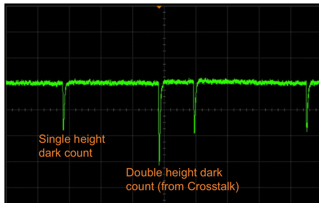
Figure 4.7: SiPM waveforms under the occurrence several dark count events. Image from [100].
