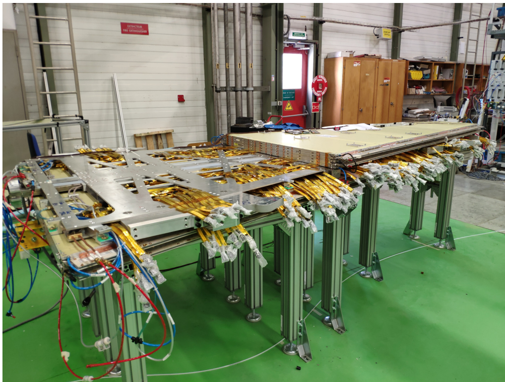
Figure 7.7: A small sector under assembly at the CERN BB5 building. The last chamber is still missing and cables to connect front-end boards are visible.
