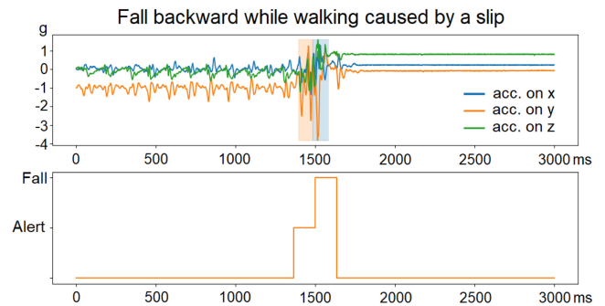
FIGURE 4. The annotation tool used to enhance the SisFall dataset. A sequence of accelerometer readings (top pane) is marked as either ALERT (in orange) or FALL (in blue). The result is translated into a time series of labels (bottom pane). The tool offers a simple mouse and keyboard interface for batch annotations.
