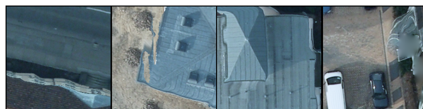
Figure 4. Example of visible distortion in RGB input images.
