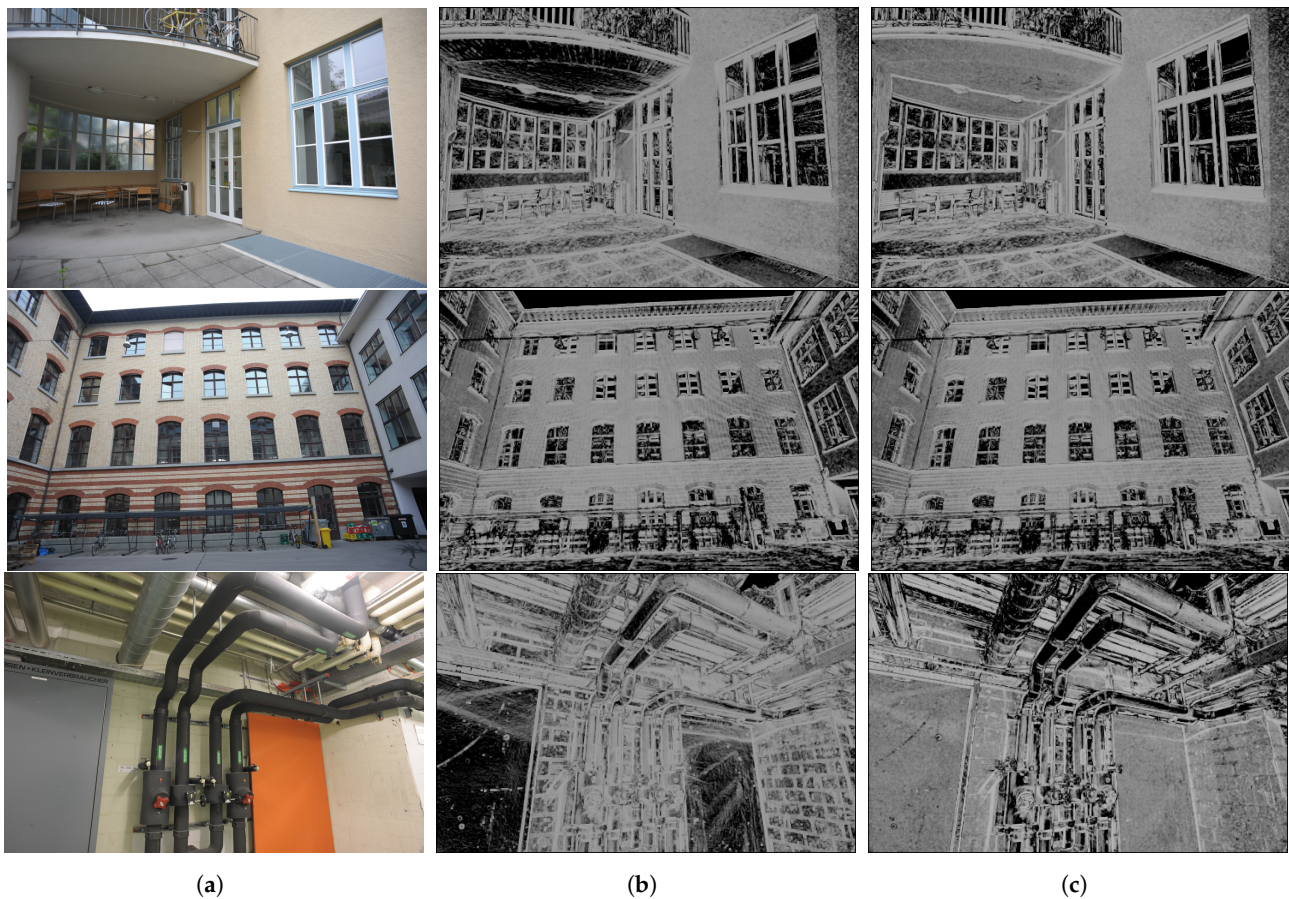
Figure 6. Qualitative confidence map comparison of our method with respect to the baseline OpenMVS on the ETH3D datasets. Scale black to white, where black means lower confidence. It is evident that the plane priors increase the confidence, especially where textureless areas are present in ETH3D-terrace (ceiling) and ETH3D-pipes (orange panel, closet). For ETH3D-courtyard where the not particularly textureless areas exist, the confidence remains mostly the same. (a) RGB image; (b) OpenMVS; (c) proposed.
