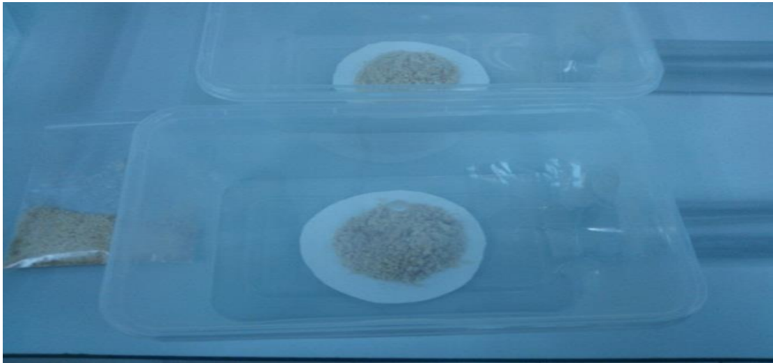
Figure 3.1: Equal amounts of Jacob's biscuit were filled into the central of the treated and untreated choice-box
