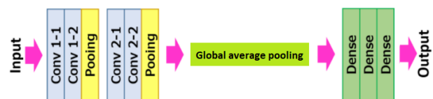
Figure 4. VGG-7 Architecture with 4 convolutional layers and a three layered fully connected one
