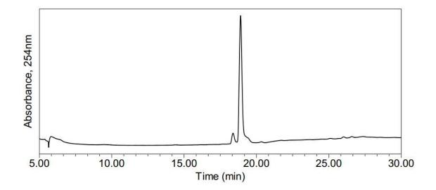
*Figure.10.* HPLC trace of TLHE Ligand 6 (>95% purity)
