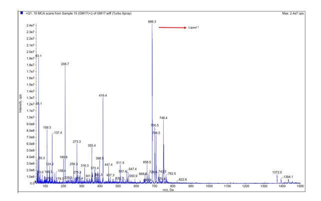
Figure.11. MS Data showing TLHE Ligand 7 (M.WT: 685)
