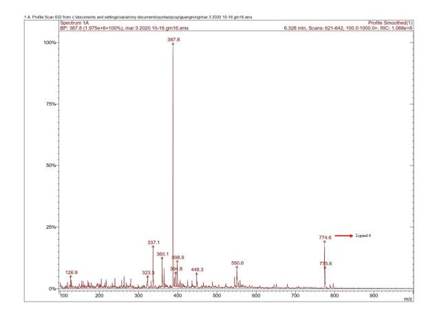
Figure 9. MS Data showing Ligand 6 (M.WT: 773.4)
