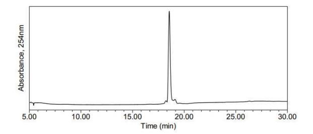
Figure 12. HPLC trace of TLHE Ligand 7 (>95% purity)
