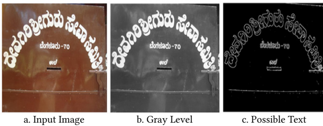
Fig. 3. Extraction of possible text component process.
