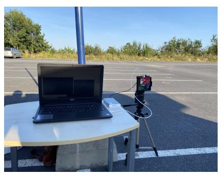
Figure 2. The mmWave radar measurement setup.
