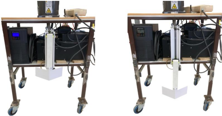
Figure 2: Figure on the left shows the marker on the module in an upright position. The figure on the right shows the marker down.
