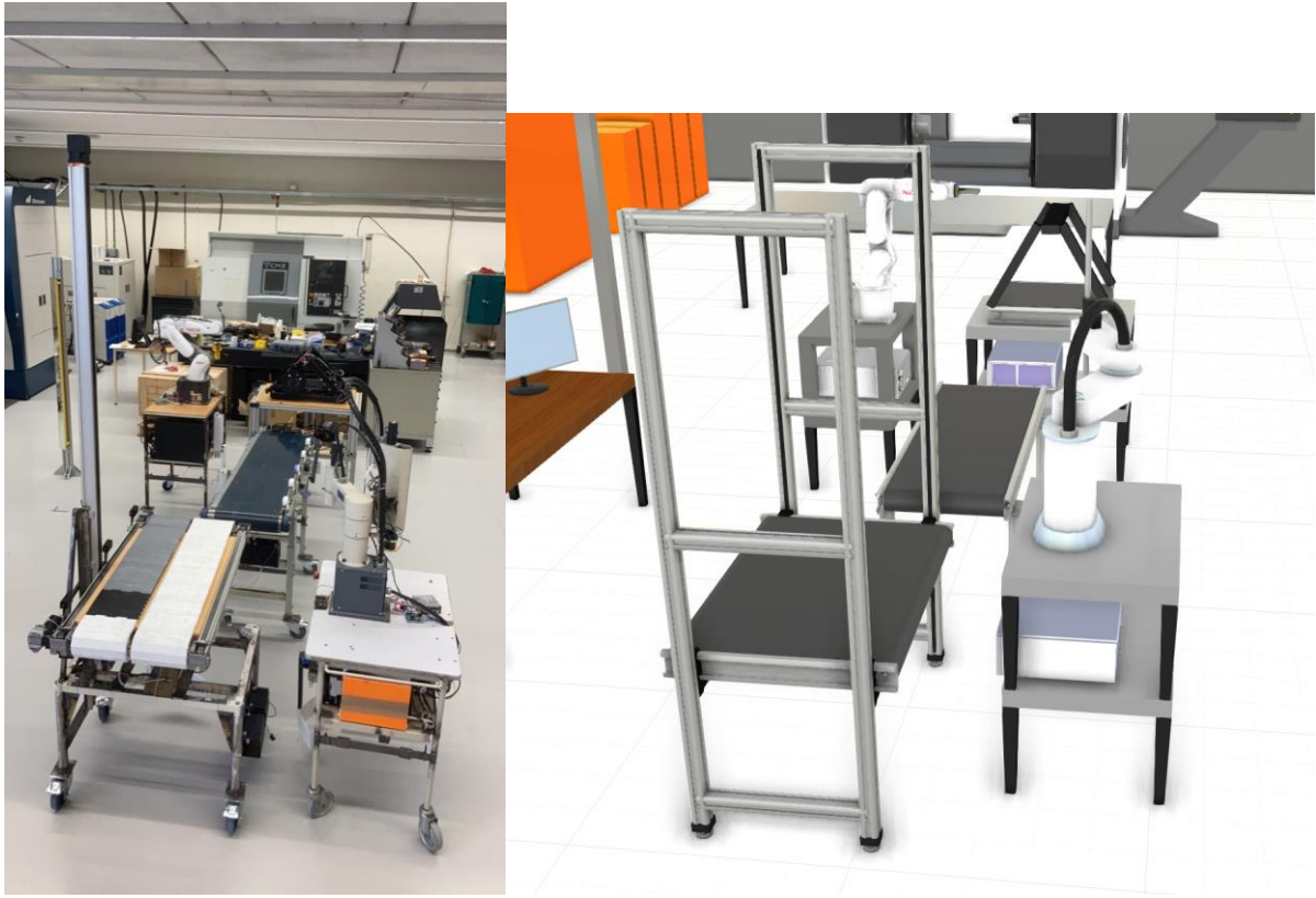
Figure 50: Comparison between the physical system (Left) and the visualization (Right).
