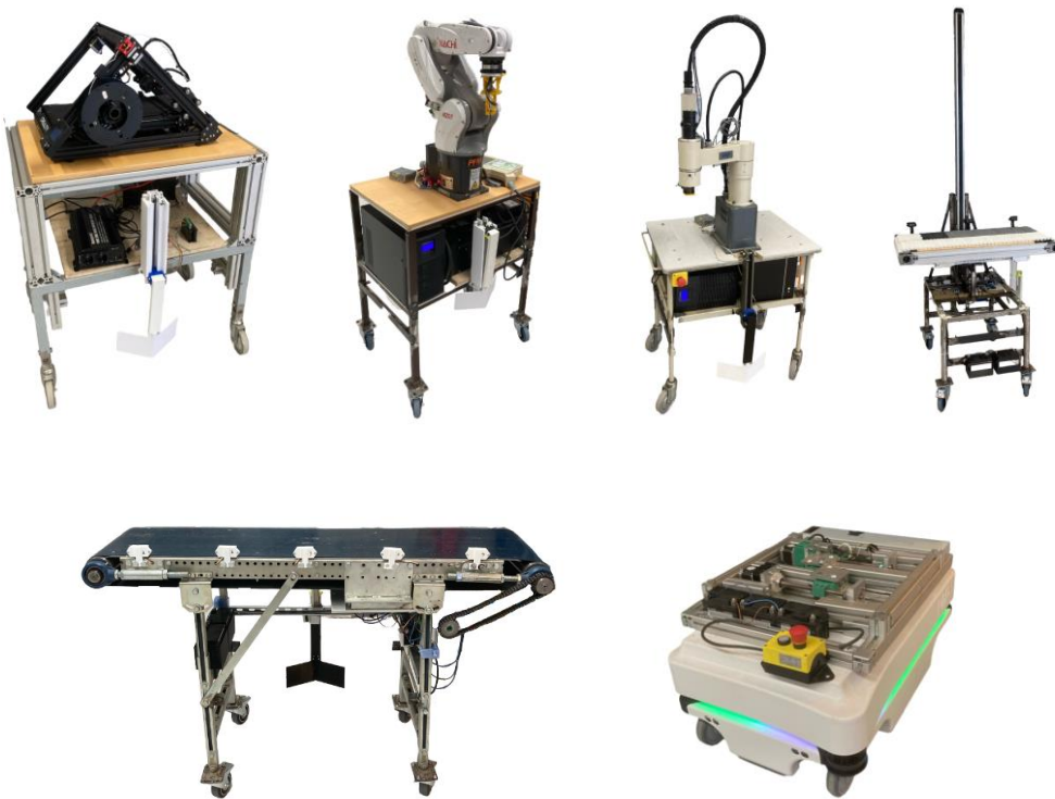
Figure 1: The five modules and the MiR-100 mobile robot that collectively represent the hardware of the RMS system.
