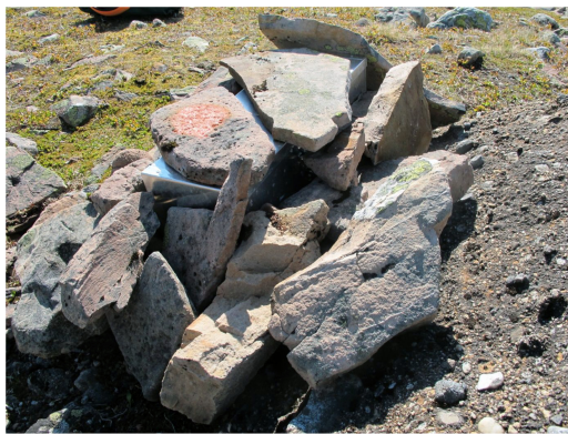
Fig. A2. Example of a camera trap embedded in a stone pile made to prevent infiltration of drifting snow that may clog the trap as shown in Fig. A1, Snow 3.
