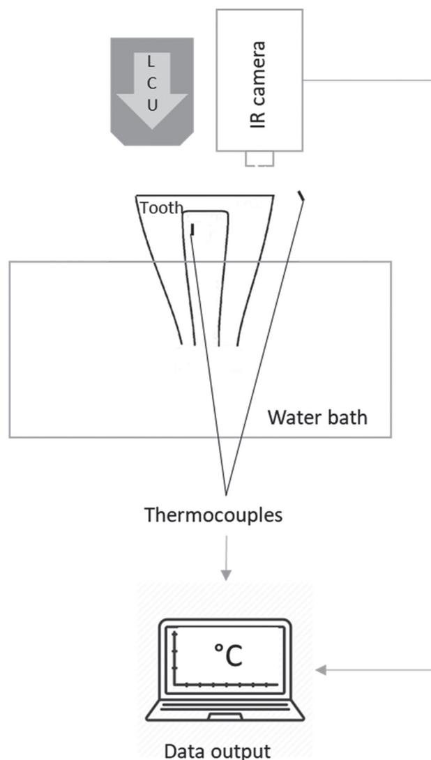
Fig. 2 Experimental setup for the measurement of the temperature development with thermocouples for the pulp chamber and infrared camera (IR camera) for the surface of a tooth when using different LED-LCU.
