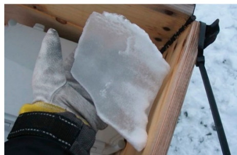
Figure 3. Ice piece thrown from a WT in Arctic Norway WF [36]. Reprint with permission from author [Matthew Homola], 2022, NTNU Norwegian University of Science and Technology.
