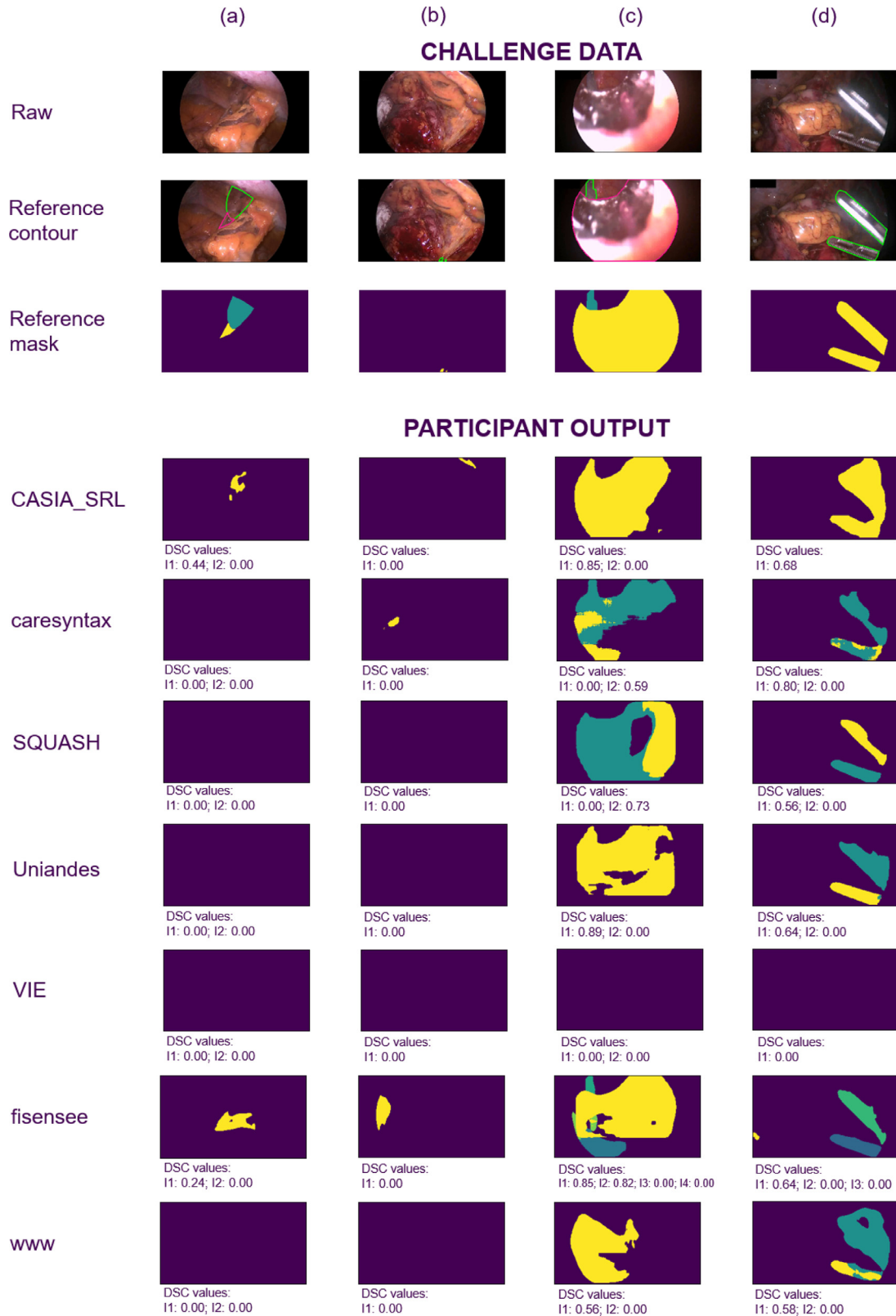
Fig. 9. Test cases with low corresponding algorithm performances. Each row shows the raw frame, the reference contours and mask as well as the algorithm output of the participating teams of the multi-instance segmentation (MIS) task for one representative frame. The columns represent image frames with (a) transparency, (b) small instruments, (c) overlapping instruments, (d) instruments near the border, respectively. For participants, the Dice Similarity Coefficient (DSC) values are provided per instrument instance ( I_i ).
