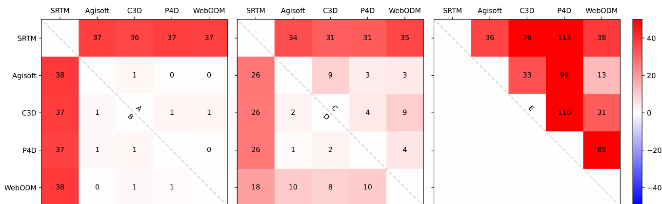
Figure 14. Root-mean-squared error (RMSE) comparison between each DSM output. The results from each dataset comprises half of the square presented, separated by the diagonal dashed line and labelled with the corresponding letter. Both columns and rows are labelled with DSM sources (SRTM and drone derived). Darker shading denotes higher RMSE values.
