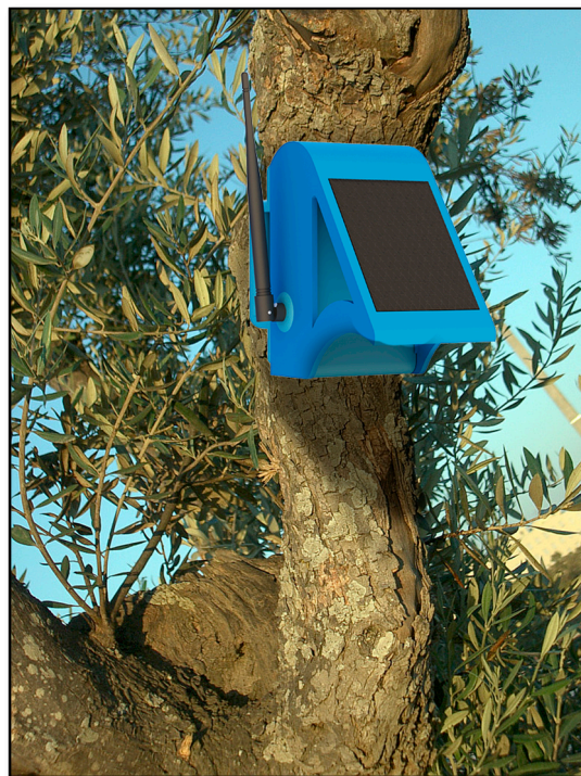
Figure 6. Placement of the monitoring device in an olive tree.
