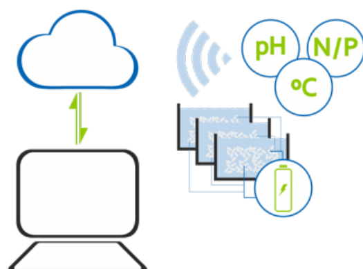
Figure 5.2 – A generic description of a wireless sensor network incorporating microbial fuel cells as a power source for biochemical sensors.
