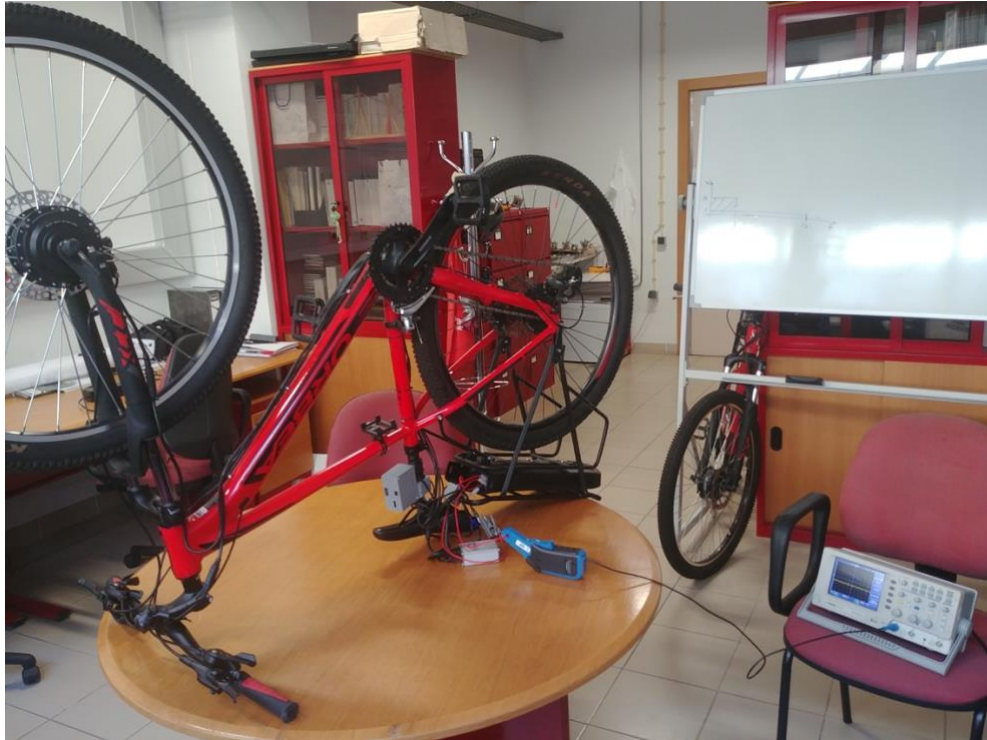
Figure 43: Experimental Setup for Test of the system in an eBike with constant current.
