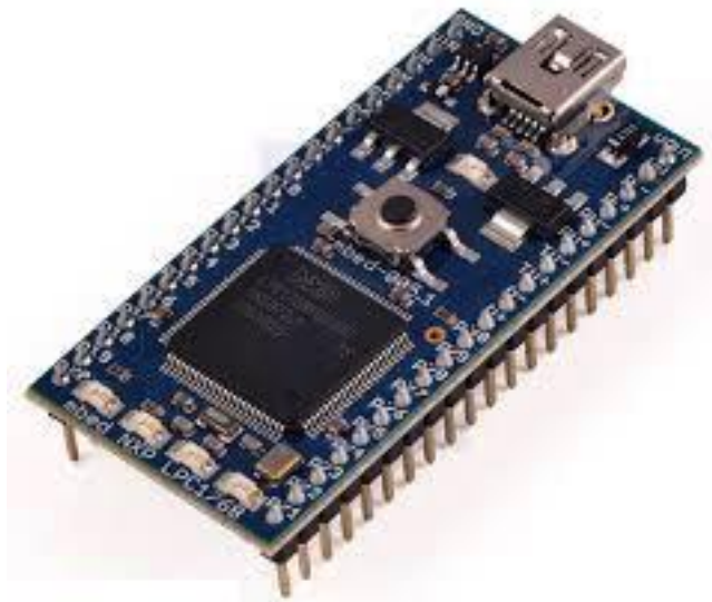
Figure 16: Microcontroller mbed NXP LPC1768.
