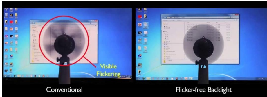
Figure 19 Flickering effects on a computer screen (BenQ APAC, 2013).
