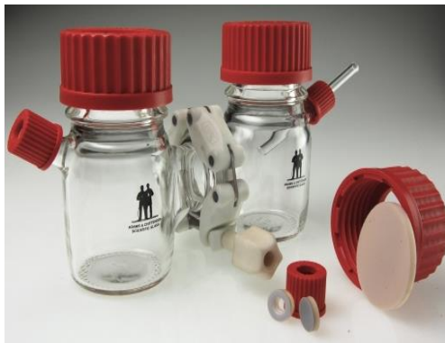
Figure 2.6: H-type MFC example
