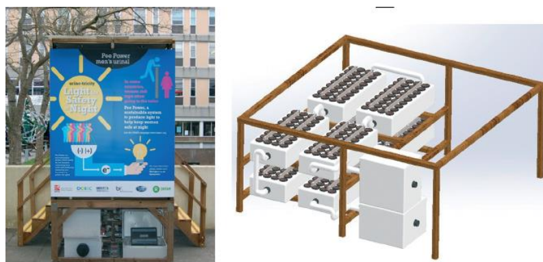
Figure 2.10: Pee power urinal at UWE campus in 2015 (from [11])
