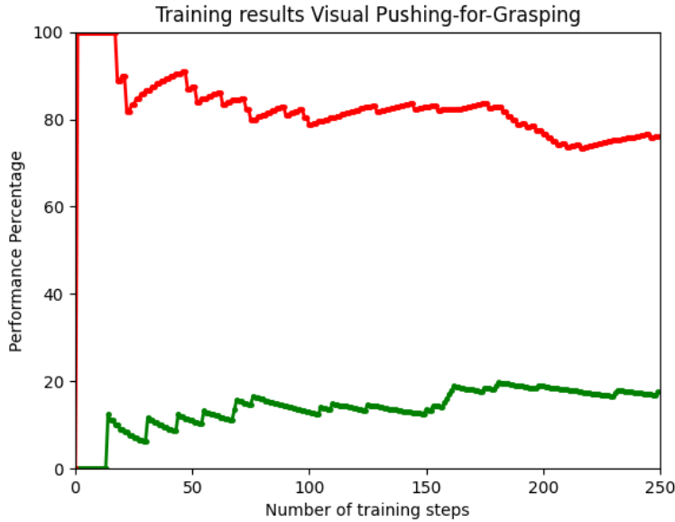
Figure 6.18: Obtained results for our adaptation of Visual Pushing-for-Grasping under 250 epochs for YCB models. In red is the Average Push to All Ratio and in green is the Average Grasp to All Ratio.
