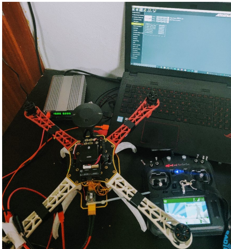
Figure 6 – Tools and connections used to calibrate the power brick.
