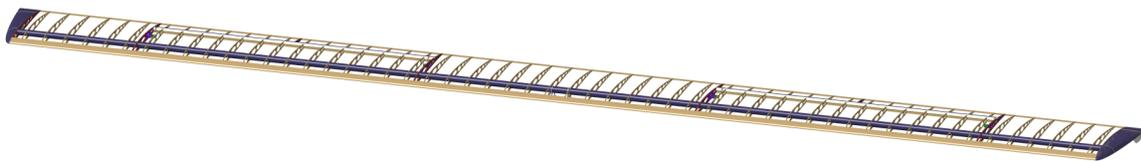
Figure 4.12: Complete wing structure without solar cells.
