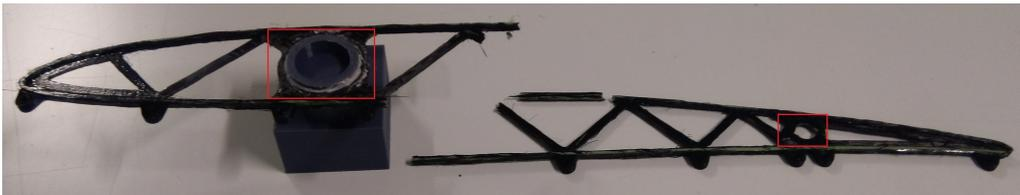
Figure 4.17: Carbon fiber sandwich rib, with a bidirectional sandwich marked by the red areas.
