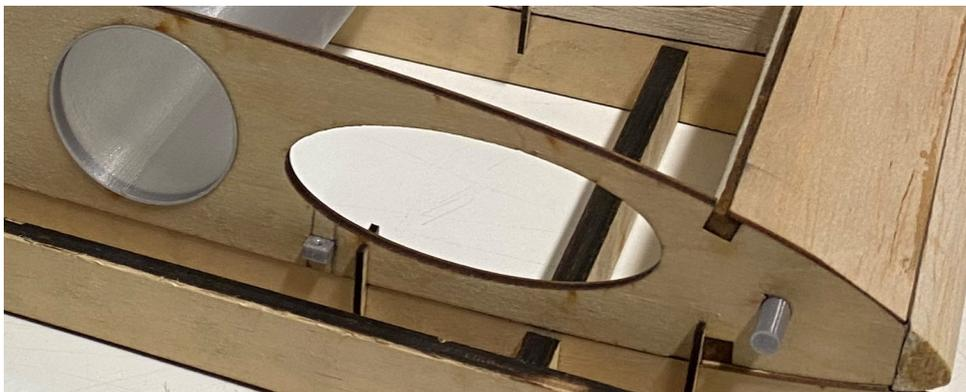
Figure 4.40: Panel torsion and axial connectors on the built wing section.
