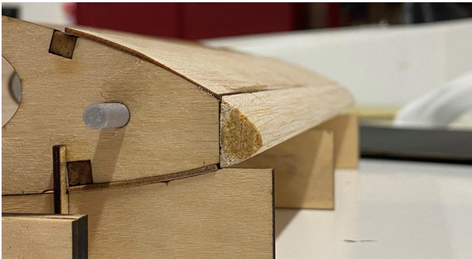
Figure 4.41: Leading edge of the built section.
