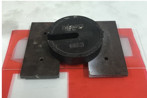
Figure 4.14: Elastomer curing process: Weights pressing a acrylic plate over the mould.
