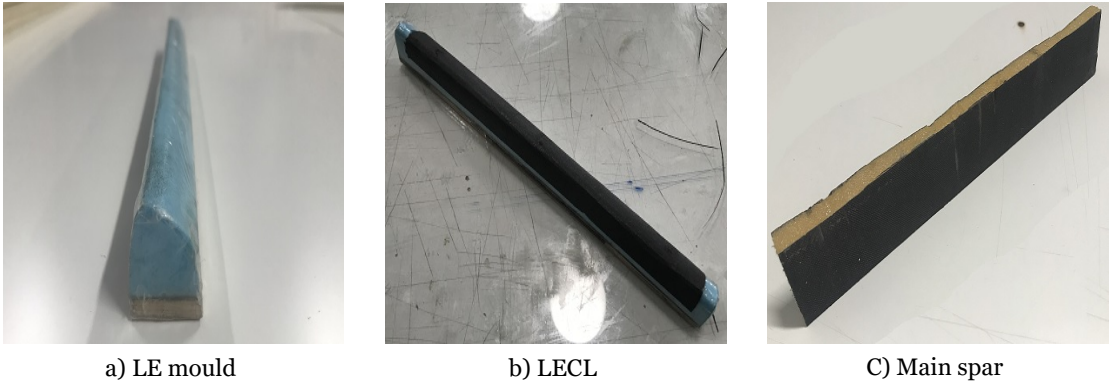
Figure 4.18: Shells LE closing laminate manufacture and main spar.
