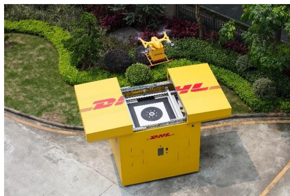
Figure 11 - EHang Falcon smart drone making a drop in an APL station. Source: [38].
