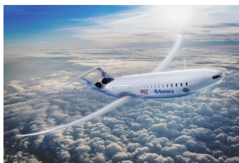
Figure 3.12: Double-bubble fuselage designed by Aurora Flight Sciences [61].
