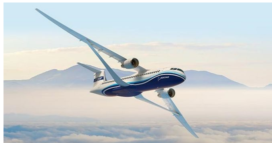
Figure 3.10: Strut-braced wing concept designed by Boeing [64].
