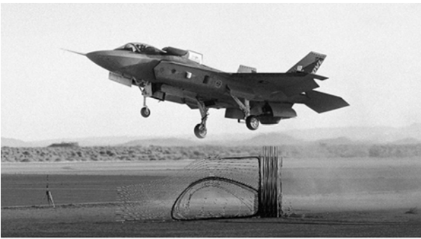
Fig. 1 Representation of the ground vortex flow phenomena on the underside of V/STOL aircrafts (Joint Strike Fighter F-35 Variant B).
