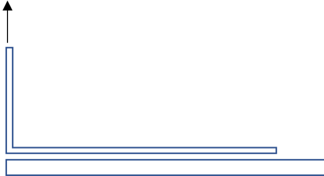
Figure 11 - Load mode typically applied in T-joint.
