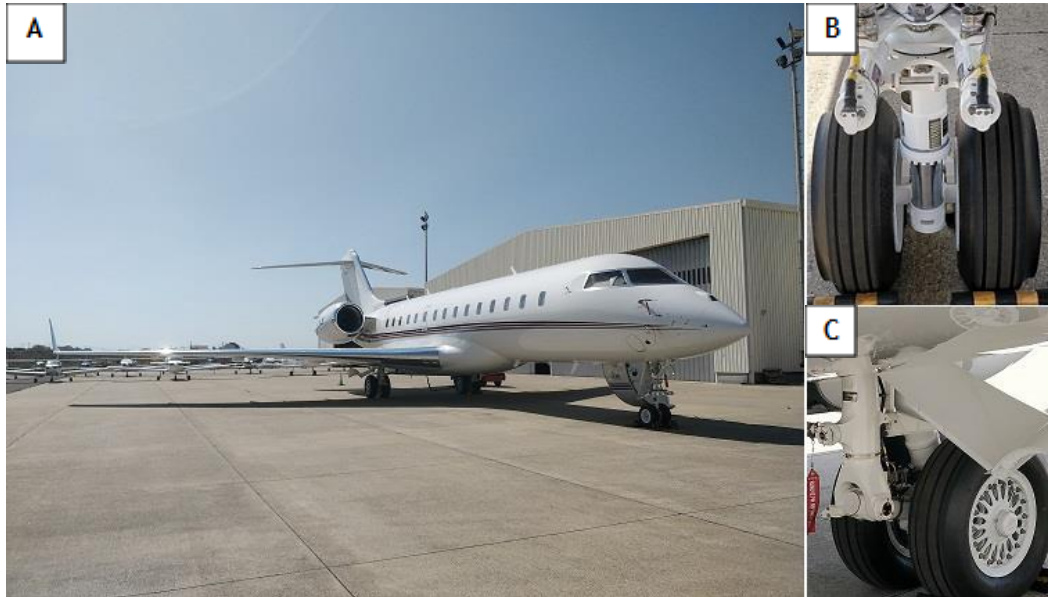
Figure 4.13: Global 6000 landing gear configuration (A - tricycle landing gear configuration; B - nose landing gear; C - main landing gear).
