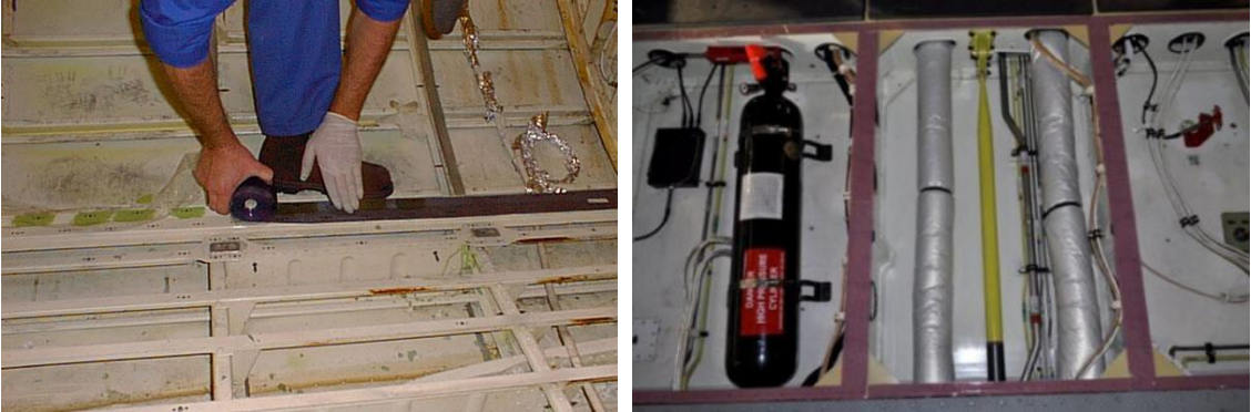
Figure 4.34: Av-DEC corrosion prevention tapes (left: HT3000; right: HT3935-7) [42, 43].
