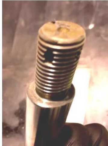
Figure 4.16: Corroded retaining bolt. (Image obtained from NetJets Europe portfolio)
