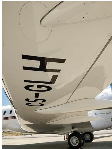
Figure 4.5: Global 6000 wing (flap tracks) fairings.
