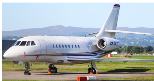
Figure 4.22: Falcon 2000ex Easy aft-fuselage engine configuration [59].
