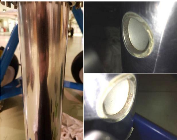
Figure 4.15: Corrosion damage found in the holes and exterior surface on the bottom part of the sliding tube. (Images obtained from NetJets Europe portfolio)
