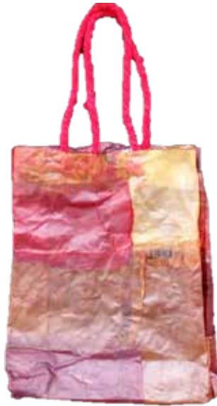
Bag made of sheets produced from fermentation of brewed tea, pulp of fruit juice and coconut water.
