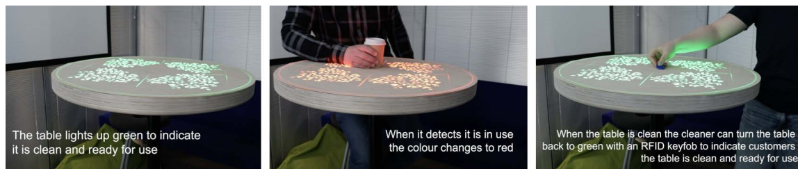
Fig. 2. CleanLeaf table use case flow (LED version)
