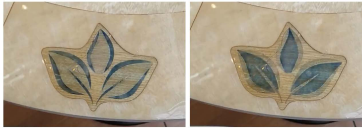
Fig. 3. The two states of the electrochromic display integrated into the table's wooden surface
