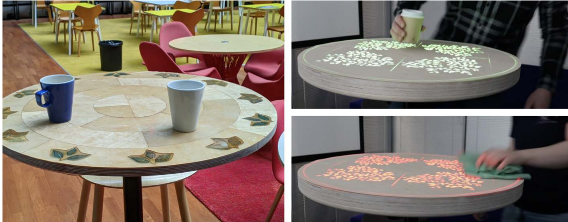
Fig. 1. The CleanLeaf table. Left: Electrochromic version. Right: LED version indicating available for use state (clean) and requiring cleaning
