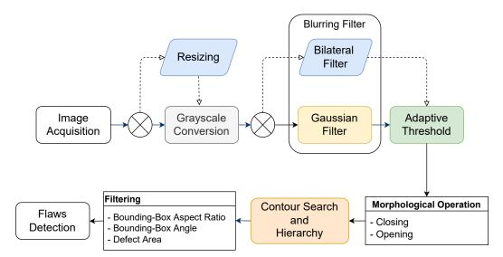
**Figure 4.** Schematic representation of the workflow of the proposed system to perform pattern analysis in the bridge inspection process.
