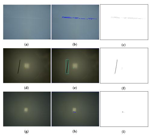
**Figure 8.** RGB images of part of the bridge under different weather conditions: sunny (**a**), night (**d**) and wet (**g**). Processed images by the flaw detection algorithm (**b**,**e**,**h**) show the colored bounding box encapsulates the flaws detected. Detected flaws are highlighted by binary images (**c**,**f**,**i**).
