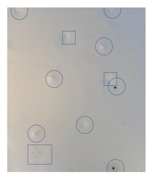
Figure 9. Result of the flaw detection algorithm performed on a 3D image.
