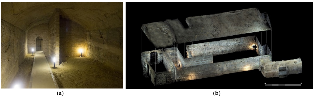
Figure 5. Sub-block 1: the “Camerone” cave (a). An exploded view of the dense point cloud obtained, in this case, with the GuPho device (b).
