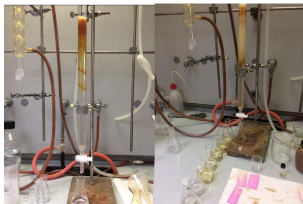
Figure 4.2 Silica gel column chromatography at the beginning of experiment (A). The fractions of mono-RL and di-RL being checked by TLC during separation (B).
