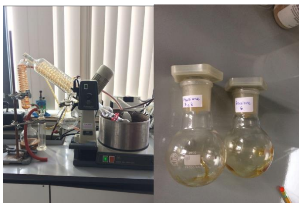
Figure 4.3 Desiccation of the fractions of mono-RL and di-RL under high vacuum
