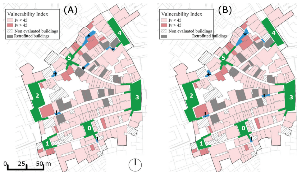
Figure 10. Oss usage for gathering purposes according to the revised evacuation plan as in Figure 4, for: A- s3 and B- s4. "Spontaneous" gathering areas are shown in blue and identified by: *, for areas similar to s1 and s2; +, for those placed near to a deleted gathering area; !, for close to a new gathering area.
