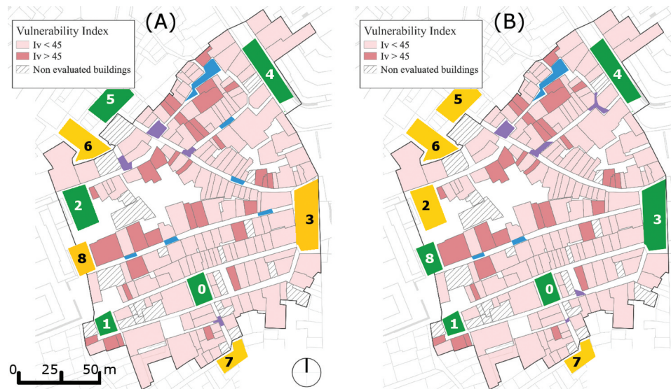
Figure 4. Oss usage for gathering purposes according to the original evacuation plan, for: (a) s1 ; (b) s2 . Gathering areas (and their accesses) are highlighted in green when Nga,perc \geq 10\% and in yellow when Nga,perc < 10\% . “Spontaneous” gathering areas are shown in blue, for those placed along the streets; in violet, for those placed at the crossroads.
