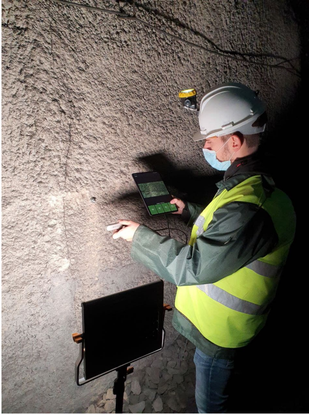
Figure 6.6: Due to the high roughness it is impossible to apply targets on the surface, therefore it is necessary to use the device equipped with a depth sensor.
