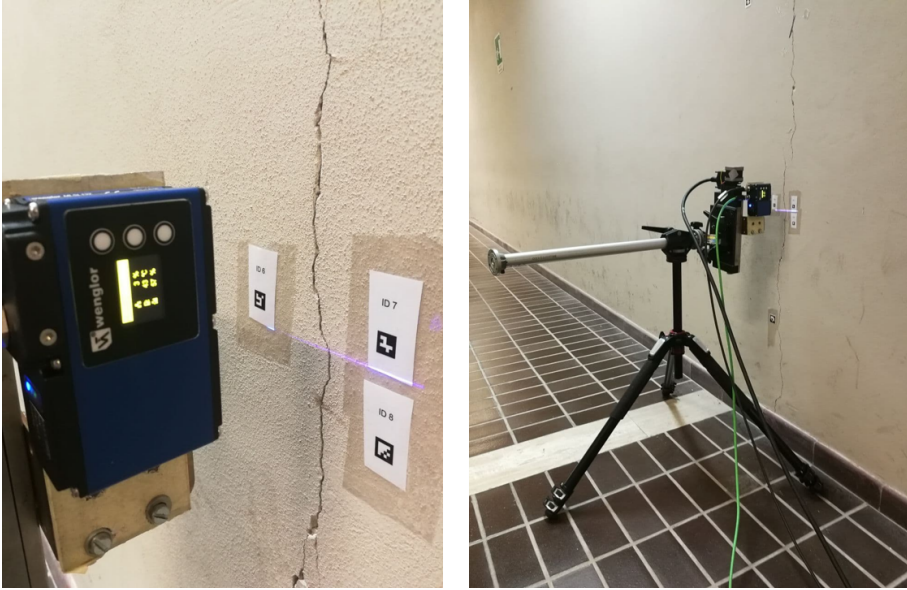
Figure 4.23: Lab-scale WENGLOR laser profilometer measurement setup.
