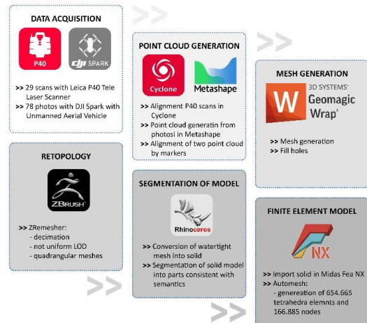
Figure 10. The workflow from Point cloud to FEA
