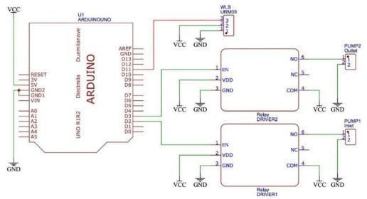
Figure 5. Schematic diagram of the hardware
