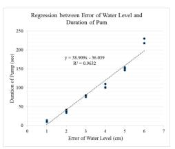
Figure 10. Linear Regression between error of Water level and the duration of pump.
