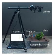
Figure 1. Image Acquisition Setup
