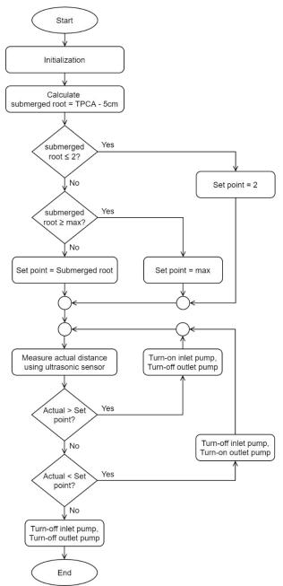
Figure 7. Flowchart of Nutrient Water Level Control program
