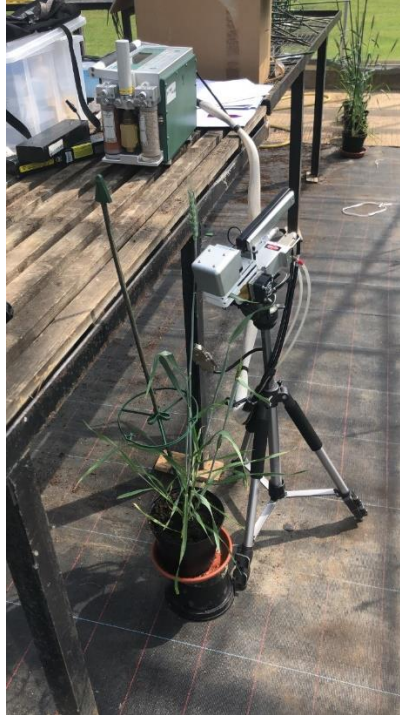
Figure 5.2. Measurements with LI-COR 6400 XT Portable Photosynthesis System in glasshouse experiment.
