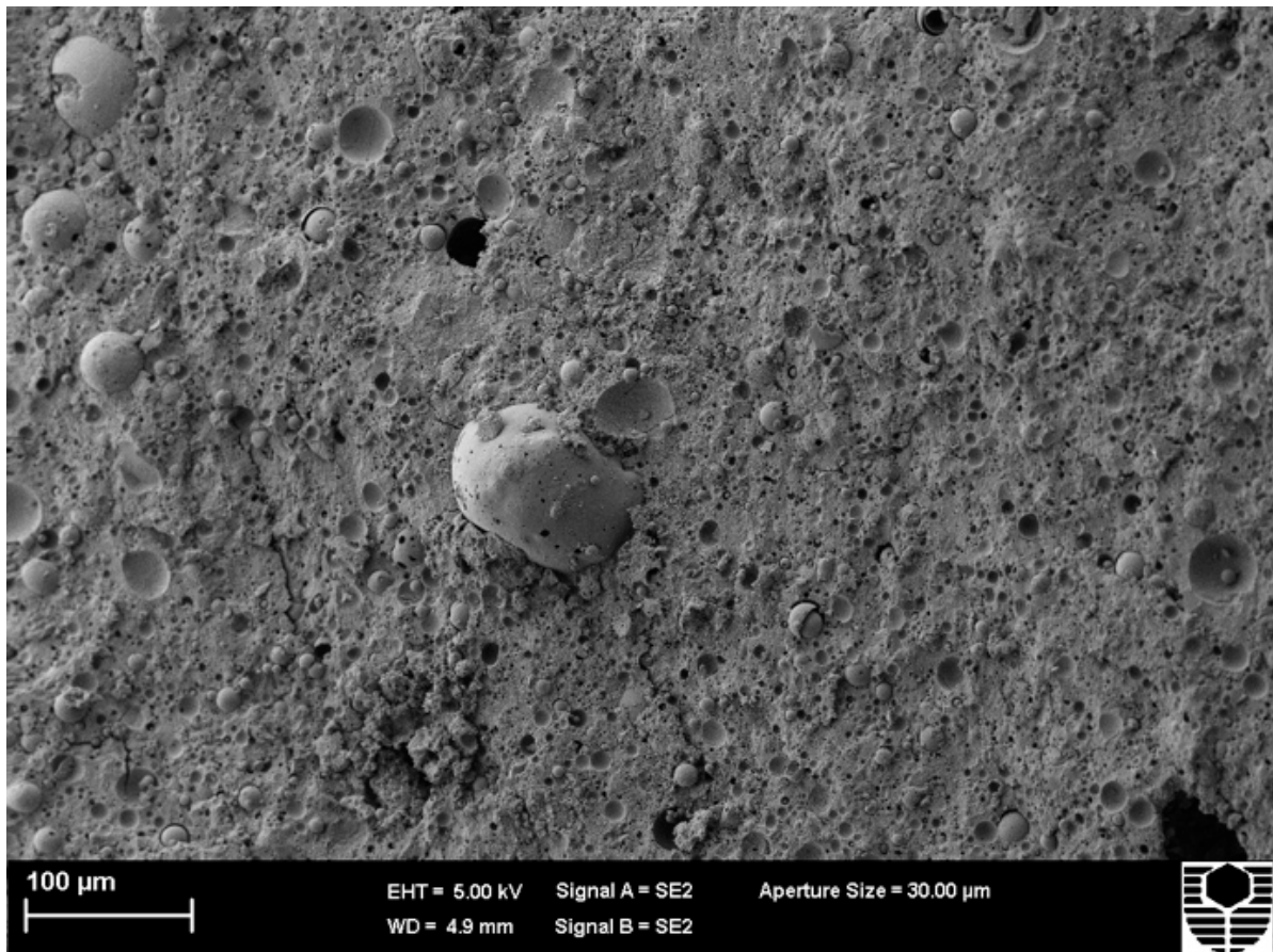
Figure 7. Microstructure of Mix 1 for FA-based geopolymer.
