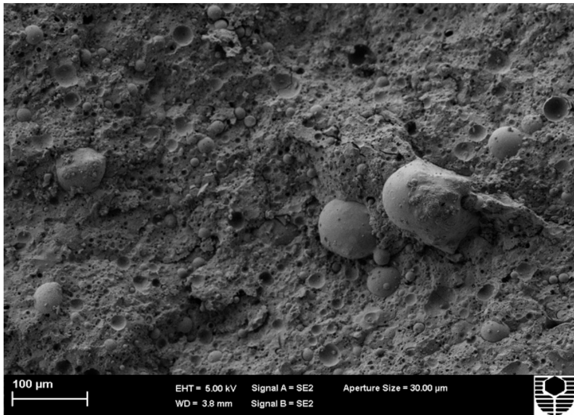
Figure 8. Microstructure of Mix 3 for FA-based geopolymer.
