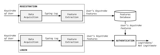
Figure 2. The overview of keystroke biometrics based on authentication system.
