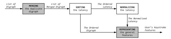
Figure 6. Block diagram of feature modeling.
