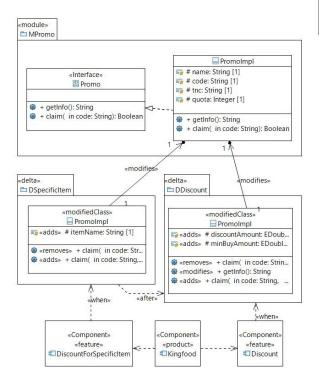
Figure 3. snippets of UML-VM diagram for restoSPL
