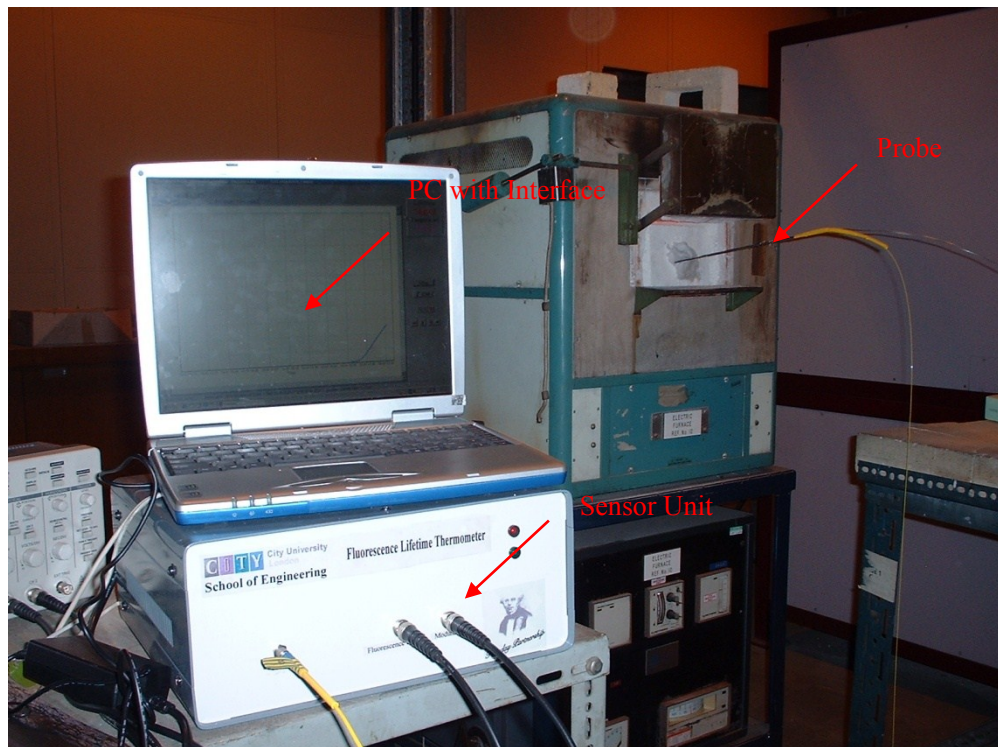
Figure 2.27: Experimental setup of the test carried out at Corus
