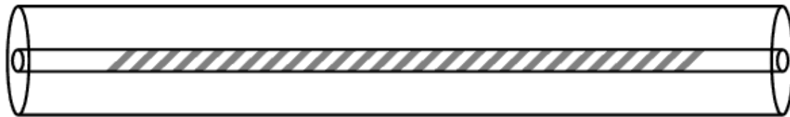
Figure 4.3: Structure of a tilted grating
