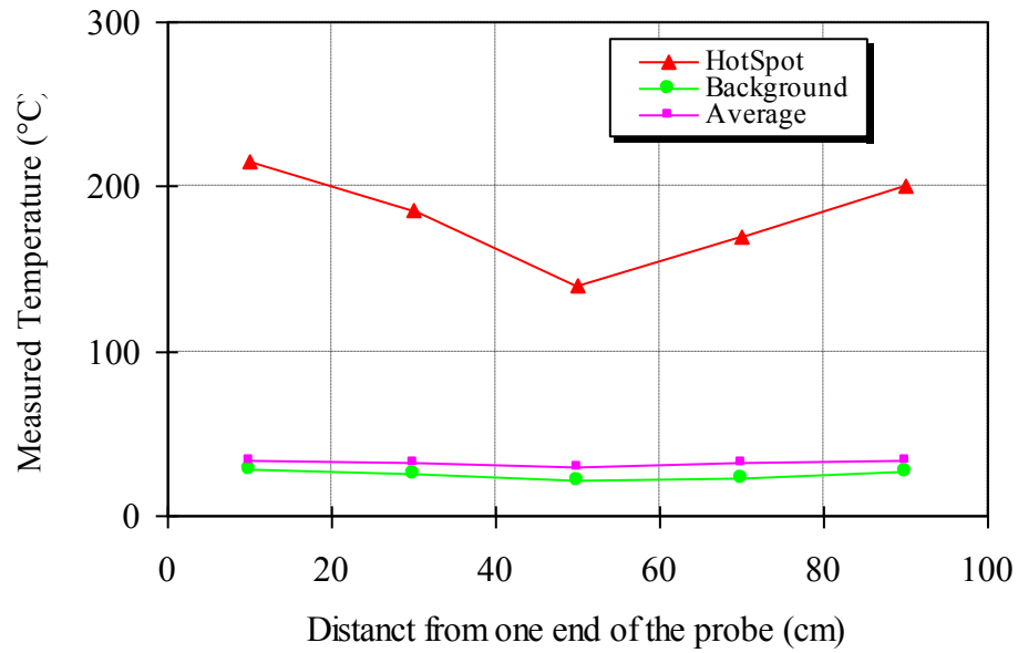
Figure 3.11: Position sensitivity of the fire alarm system (At room temperature background and 200°C hotspot)
