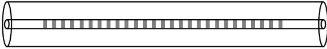
Figure 4.2: Structure of a uniform fibre Bragg grating
