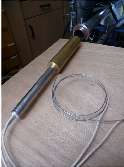
Figure 4.18 Cartridge heater components
