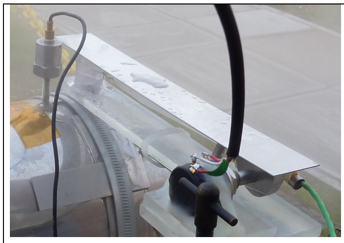
Figure 6.9 Air flow meter using metal flap
