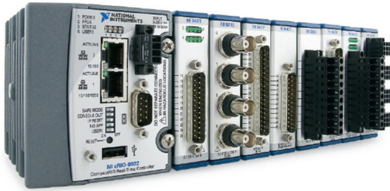
Figure 6.1 CompactRIO™ with 8 module chassis (picture courtesy of National Instruments (2009a))
