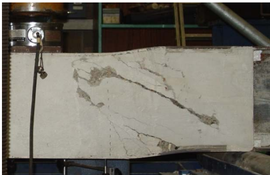
Figure 9. USFB No.3 at Failure point.
