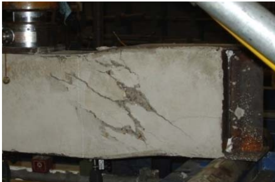
Figure 7. USFB No.1 at Failure point.
