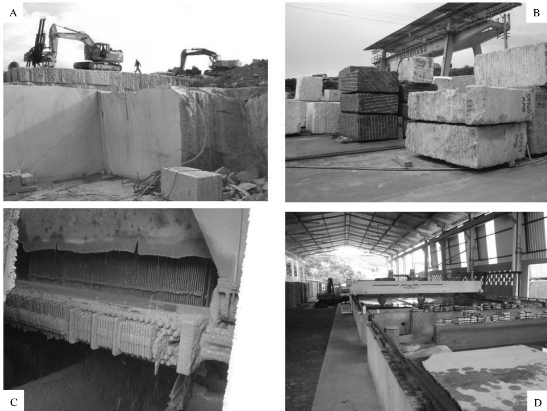
Figure 2. Pictures showing a typical quarry, saw and polishing place. In the places where the waste material is deposited the water content lowers from 80% to 20%. A. Quarry; B. Deposit of blocks; C. Saw; D. Polishing process.
