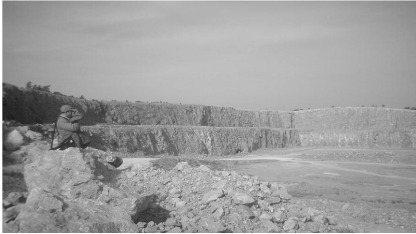
Figure 2. Limestone aggregates Quarry from Slovenia, which uses strip banded method.
