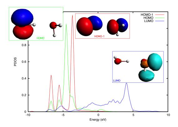
**Fig. 1** Density of state of the water dimer adsorbed at a Rh(111) surface projected on the HOMO-1, the HOMO and the LUMO orbitals of the water dimer. The corresponding orbitals are represented close to the corresponding peak density: in green, left handside, the HOMO; in red, middle, the HOMO; in blue, right handside, the LUMO.
