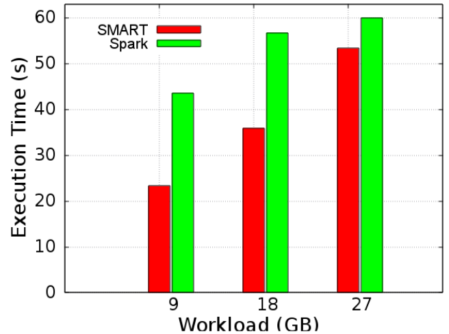
Figure 5. SMART vs. Spark streaming execution @ wordcount
