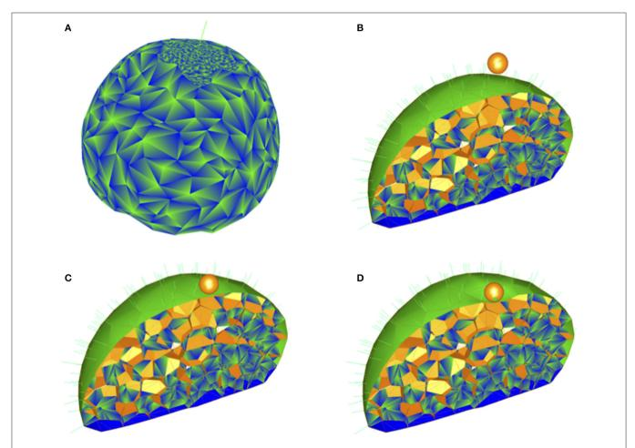
FIGURE 1 | Indentation of a three dimensional plant tissue by a spherical probe. (A) Outer view of the triangular mesh, showing the refinement of the mesh at the indented cell and its neighbors. (B–D) Spherical probe and views of sectioned simulated flower bud before contact between probe and tissue (B), at the first contact (C), and at maximal displacement (D). The colors were chosen to help visualization of facets and types of facets.
