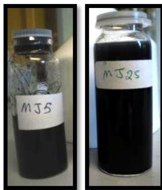
Fig.15. Photograph of MWCNTs2 after mixing with hairy Janus particle SET-151 in experiment (MJ5), and with hairy Janus Particles SET-163 brushes in experiments (MJ25).
