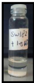
Fig.31. Photograph of the phase separation that occurred when patchy particles (SW-182) with poly[2-methacryloyloxy ethyl]-trimethyl ammonium chloride] (MAETAC) brushes were used.
