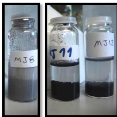
Fig.2. Photograph of phase separation of MWCNTs2 in experiments (MJ8, MJ11) after mixing with anionic spherical latex particles, and phase separation of SWCNTs in experiment MJ12.
